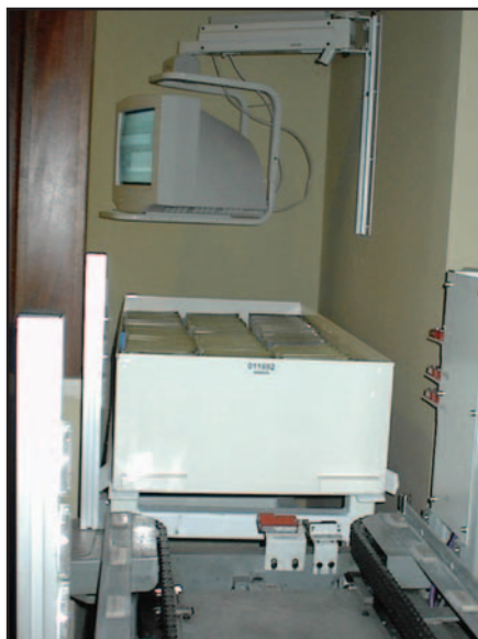
After requests and work orders are generated in the ARS, 4-foot-by-2-foot metal carriers are retrieved from the vault's rack and delivered to operators at the "pick-and-delivery" stations.
