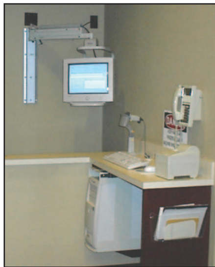
Operators process the arrival of carriers at one of Steelcase Library's three operator stations and follow instructions on the screen to identify and retrieve the correct items.
