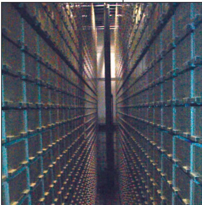
At 100 feet long, 15 feet wide and 40 feet high, the vault in the Steelcase Library's automated retrieval system can hold up to 250,000 volumes.
